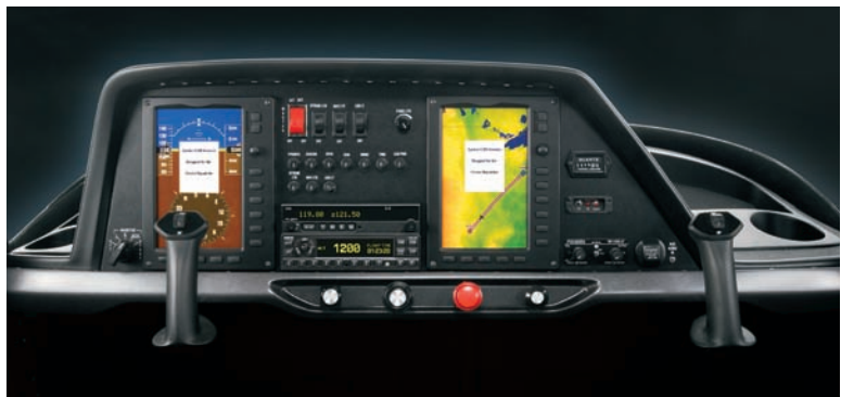
Garmin G300 glass cockpit designed specifically for the Cessna Skycatcher.
